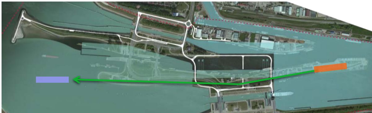
Figure 12. Cutter dredger (indicated location in orange) transporting its dredged soil via the green floating lines/land lines/bridges (Figure 11) to the barge (indicated location in purple) waiting in the outer harbor. The purple barge will sail direction of the Westerschelde/Knokke-Heist for disposal of dredged material.
